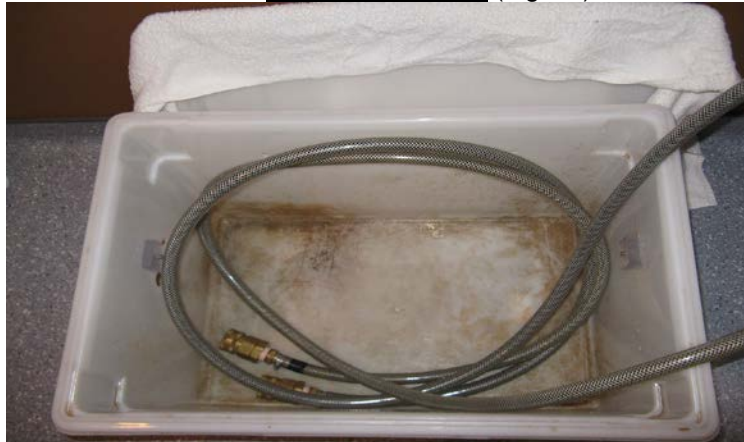
Figure 10. Water Switch Box opened. Store box lid behind the box.
