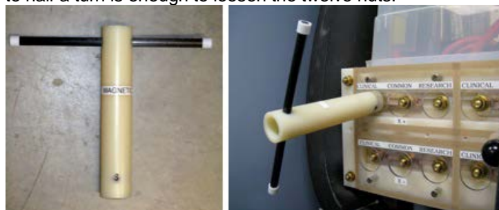
Figure 16. Use the tool shown at the left to loosen the brass nuts.
