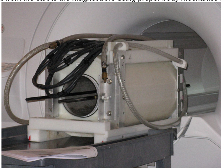
Figure 8. Alignment of insert coil and bore of the magnet
