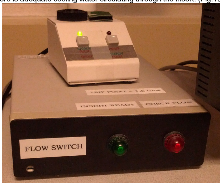
Figure 19. Flow monitoring device. Power switch is located on the back.
